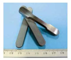
These metallic bar and dog-bone sample specimens are used to characterize behavior through tensile testing.
