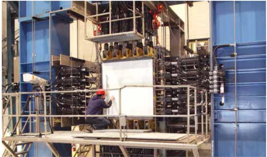
The system upgrade also included an entirely new hydraulic distribution system, comprising two SilentFlo™ hydraulic power units, a Model 293 Hydraulic Service Manifold, and integrated hard line.
