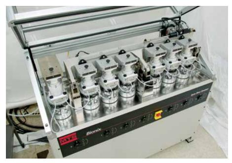
The Bionix Spine Wear Simulator features six active specimen containment modules to provide a statistically valid sample size.
