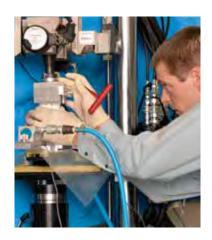
"We find the multiaxial system especially useful for spine kinematics studies, because we can test in multiple directions simultaneously. Combining flexion, extension, bending and torsion at the same time allows us to simulate the full range of motion in a highly realistic manner, without spending time on stopping and readjusting."
