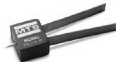
Standard equipment includes the gage and storage case, two reusable hardened knife edges for attachment to the specimen, and an instruction manual.
