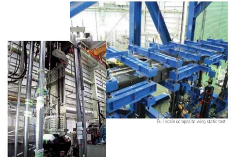
Composite subcomponent fatigue test
