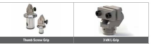
There are several different tensile grips that can be used for ISO 6721-4. The easy-to-use, 3 kN Thumb Screw Grip works well for smaller specimens. The MTS Toggle Grip (not pictured) is self-tightening so it maintains the most consistent clamp load throughout the test. The MTS L-Grips are economical and come in both 250 N and 3 kN capacities.
